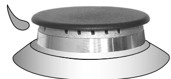
Excessive lift off, usually due to pressure too high
