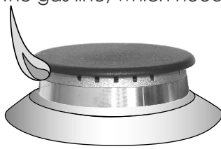
Excessive yellowing, usually due to insufficient oxygen
