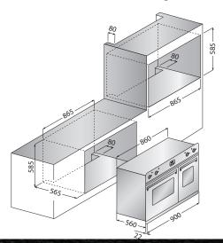
Model D900 WMP Total electrical load 4.9 kW Cut out - hole dimension: 585mm x 865mm
