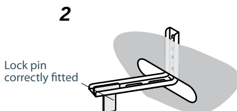
Fig. 18c Fitting the lock pin through the bracket
