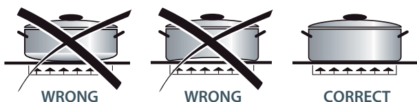
Fig. 74 Inefficient and efficient saucepan bottoms
