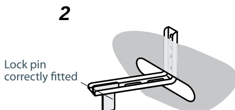
Fig. 6c Fitting the lock pin through the bracket
