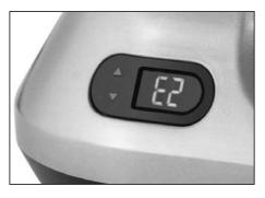
If this error occurs, turn the speed control dial to the 'Off' position, switch the appliance off at the power outlet and unplug the cord. Wait at least 15 minutes before restarting the mixer.
