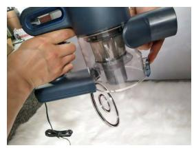
To take out the HEPA filter: Either turn it by hand, then take it out or use the nozzle to help if needed.
