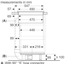
A: With 90° "S" bow connector B: With 90° "L" bow connector
