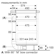
A: With 90° "M" bow connector B: With 90° "L" bow connector
