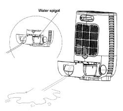
3. The other end of this hose must be placed over a water drain.
