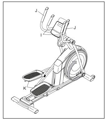
To dismount the elliptical, wait until the pedals (K) come to a complete stop. Note: The elliptical does not have a free wheel; the pedals will continue to move until the flywheel stops. When the pedals are stationary, step off the higher pedal first. Then, step off the lower pedal.
