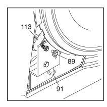
When the drive belt is properly adjusted, reattach the parts that you removed. Then, plug in the power adapter.
