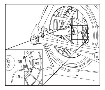
Next, slightly loosen the indicated two M4 x 13mm Self-tapping Screws (50). Slide the Reed Switch (38) slightly closer to or away from the Magnet (43), and then retighten the Self-tapping Screws.
