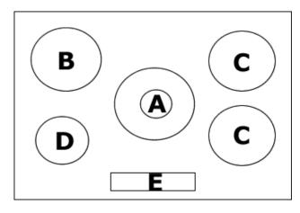
**A** = 3.80 kW triple crown (wok) burner
