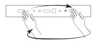
To decrease the fan speed, wave your hand from right to left, reducing the speed from 3 - 2 - 1 - 0. The current speed setting will be shown on the screen.
