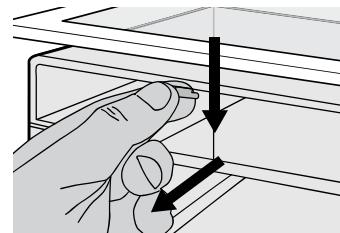
3. Remove the centre runner by disengaging it at the front of the shelf, and removing it from the rear.
