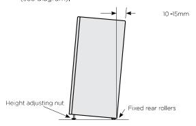
3. Wind the large height adjusting nut on the handle side down until the refrigerator is level and stable. If you have difficulty winding the nut or height adjusting foot down, have someone tilt the refrigerator back so you have better access.
