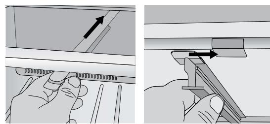
Insert into the slot at the rear of the shelf      Then engage into the front of the shelf
