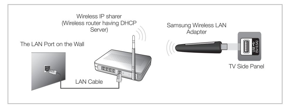
Samsung's Wireless LAN adapter is sold separately and is offered by select retailers and Ecommerce sites. Samsung's Wireless LAN adapter supports the IEEE 802.11a/b/g and n communication protocols. Samsung recommends using IEEE 802.11n. When you play video over a network connection, the video may not be played smoothly.
