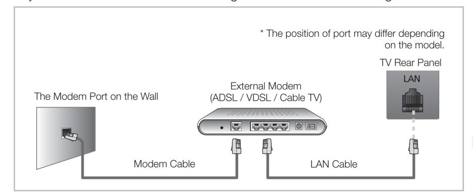
You can attach your TV to your LAN by connecting the LAN port on the back of your TV to a IP Sharer which is connected to an external modem. Use LAN cable for the connection. See the diagram below.
