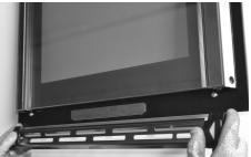
4. Slide out the internal glass as shown below. Remove the second and third panes of glass (middle panes) for cleaning sliding out the rubber strip.
