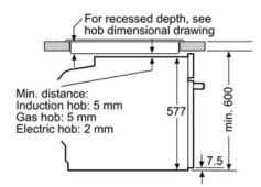
measurements in mm
