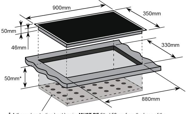
\* A <u>thermal protection heat barrier</u> **MUST BE** fitted 50mm from the base of the cooktop when access is possible via a cupboard or drawer. This thermal protection heat barrier should contain holes to improve ventilation as shown.
