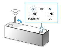
When the Wi-Fi connection is complete, the LINK indicator lights up in green.
