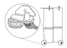
Open the door and use the spanner ● to loosen the keeper nut by turning it to the left.
