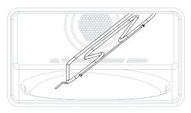
Remove the grill resistor by pressing on the rod in the upper left.
