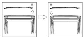
8 Install the upper door, fix the upper door hinge onto the cabinet.
