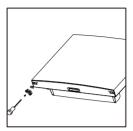
Use a flat-bladed screwdriver to pry open the upper door sleeve and corner plastic cover. Turn the door sleeve 180° then put it back on the upper door.
