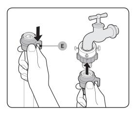
**6.** While holding down part (E), connect the water hose to the adaptor. Then, release part (E). The hose fits into the adaptor with a clicking sound.
