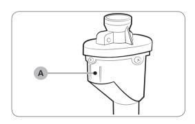
The aqua hose alerts users of a risk of water leaks. It senses the water flow and turns red on the centre **indicator (A)** in case of a leak.
