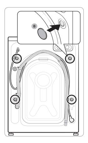
**3.** Insert the **bolt caps (B)** to the holes (marked with circle in the figure).
