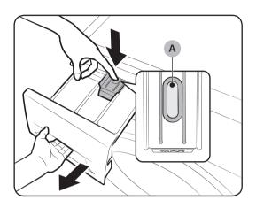
**1.** While holding down the release lever inside the drawer, slide open the drawer.
