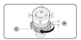
**3.** Holde the adaptor and turn part (C) in the arrow direction to loosen it by 5 mm (\*).
