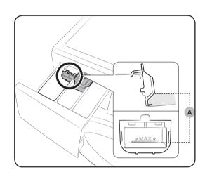
First insert the provided liquid detergent container in the II main-wash compartment. Then, apply liquid detergent to the container below the marked max line (A).
