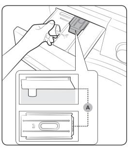
**3.** Apply fabric softener to the **softener** compartment. Do not exceed the max line.
