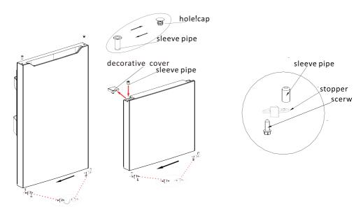
**Step 5** Install the refrigerator compartment door on the lower hinge, then install the middle hinge and hole caps.
