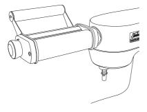
2.Set adjustment knob on pasta roller at 1 by pulling the knob straight out and turning to setting 1. The numbered graphics are shown on the knob. Release knob, ensuring the knob locks in place, against the roller housing.
