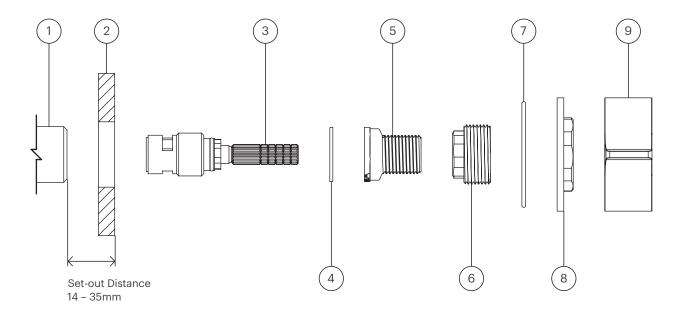
Note: For Retro-fit installations, make sure the set-out distance is within the range stated before commencing any work.
