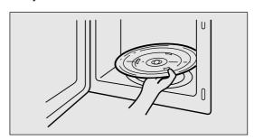
7. The roller guide and oven cavity floor should be cleaned regularly to avoid excessive noise. Simply wipe the bottom surface of the oven with mild detergent water or window cleaner and dry. The roller guide may be washed in mild sudsy water.
