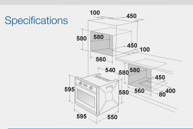
Product Dimensions: H595 x W595 x D550mm Cut-out size (proudmount): H580 x W560 x D580mm Cut-out size (flushmount): H598 x W598 x D580mm 220-240V - 50Hz
