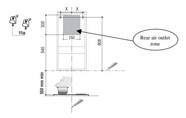
When installing the hood in recycling version it has to be taken into consideration that space remaining between the hood and the upper limit (ceiling or self) is at least 8-10 cm.
