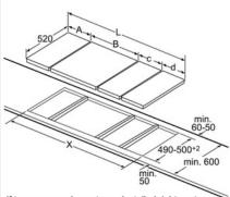
If two or more elements are installed right next to one another, one or several installation kits are required (2 elements 1 installation kit, 3 elements 2 installation kits, etc.).
