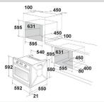
**Product Dimensions:** H592 x W592 x D571mm Cut-out size (proudmount): H582 x W582 x D600mm Cut-out size (flushmount): H595 x W595 x D631mm
