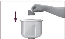
4. Align the D shaped hole on the paddle with the D shape on the drive shaft inside the bread pan. Push down firmly. The paddle should rotate with the drive shaft. It is important that the paddle is properly assembled onto the drive shaft to ensure ingredients are mixed and kneaded properly.
