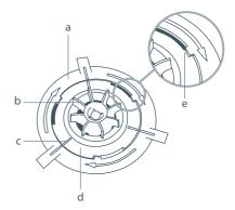
Correct locking position of filter plate with motor assembly (under spray arm)
