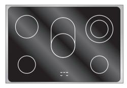
The appliance has 5 cooking zones of various diameters and power levels. Their position is clearly indicated with circles and heat is released within the diameters traced on the glass ceramic surface. The 5 cooking zones are HIGH-LIGHT zones and come on a few seconds after activation. The heat intensity can be adjusted using the knobs
