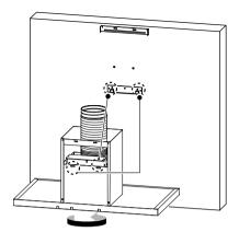
6 After connecting the exhaust pipe securely, fix the chimney fixing bracket with 2 screws with prepared wall plugs to prevent the appliance from accidentally sliding off the hood fixing bracket.
