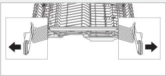
Pull out the top cutlery tray. Press the top spray arm up and unscrew the spray arm bearings counter-clockwise to remove the spray arm.
