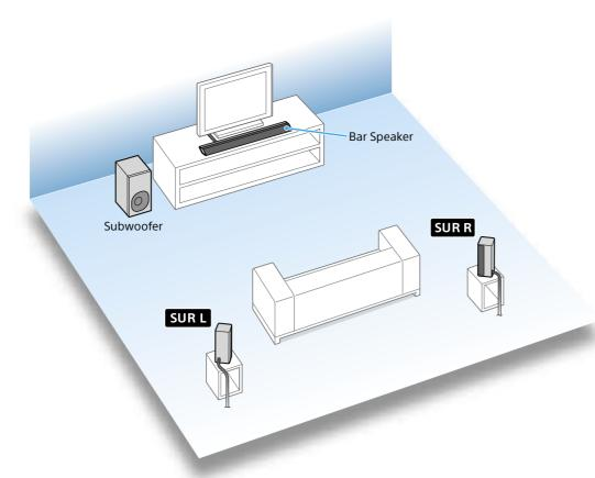
• There are the labels on the rear of the each speaker. Make sure to identify "SUR L" (left) and "SUR R" (right) and place the speakers in the correct places.
