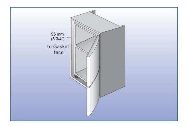
Lift the front edge of the product and slide the integration foot under the levelling foot. Push the product back to allow the outer cabinet door to close. This will be approximately 95mm (3 3/4") from the front edge of the built in cabinet to the gasket face of the refrigerator.
