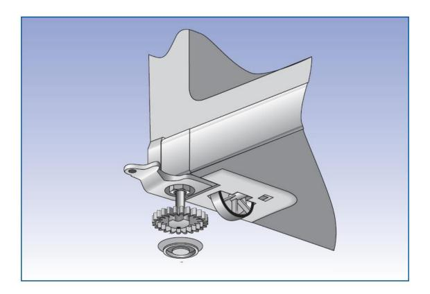
Tilt the product back and remove the levelling foot circular base insert from the front levelling feet, a small flat blade screw driver can be used.
