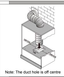
Connect the hose (not supplied) to the damper flap and place the duct hose into position.
