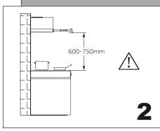
Install the hood no less than 600mm and no more than 750mm above the cooking surface.
