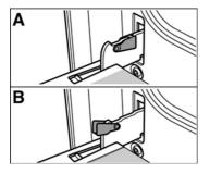
The hinges of the appliance door are each secured by a locking lever.
