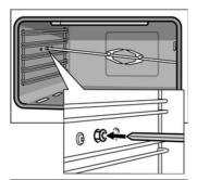
2. If the oven has been preheated, only attach the rotary spit if you are using an oven cloth or wearing (thermal) oven gloves. To attach the spit, slide one end into the recessed adapter in the left-hand side panel of the cooking compartment.
