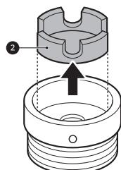
3 Push the adapter onto the end of the tap so that the rubber seal is connected to be watertight. Tighten the 4 fixing screws.
