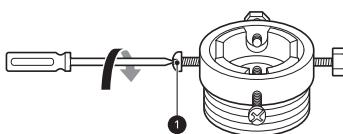
2 Remove the guide plate ② if the tap is too large to fit the adapter.
