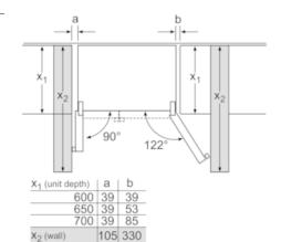
measurements in mm
