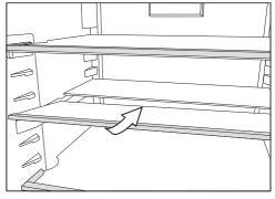
■ Lift up the front section of the glass shelf slightly at the front and slide it carefully underneath the rear section.
