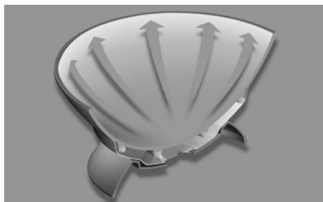
Heat-Wall element channels heat upwards
