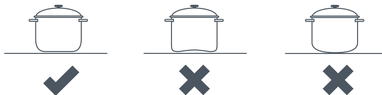
Fig.10 Efficient and inefficient saucepan bottoms
