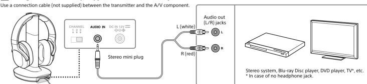
If the sound is distorted by connecting the transmitter to the A/V component's audio out (L/R) jacks, reconnect the transmitter to the headphone jack. If the transmitter detects no signal or no sound, check the connection of the connected A/V components, then check the audio setting of the connected A/V components.
