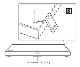
Operate the system with the display of the Android device.
