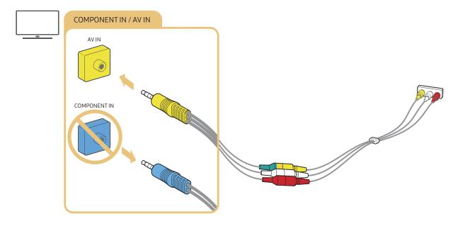
Connect AV (composite) equipment to AV In only. Do not connect to Component In.
