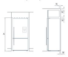
Flush with refrigerator chassis – full door rotation
