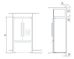
Flush with refrigerator chassis – full door rotation
