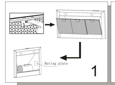
Check voltage and Frequency given on the rating plate located on the inside of the hood.
