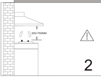
We recommend that after installation the bottom of the hood should be no less than 600mm and no more than 750mm above the stove's heating elements and burners.
