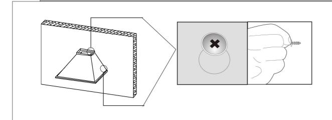
Screw down the four screws, first screw down the upper two screws, then screw down the other two screws.
