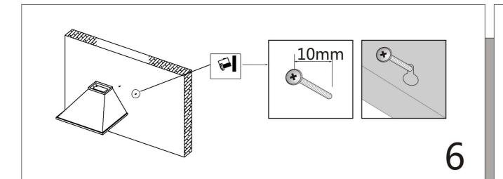
Hang the hood and let it's 4 installation holes aim at 4 screws, adjust it to setting position.
