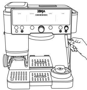
**NOTE:** When the machine is out of water, it will not purge. Be sure to press the PURGE button when adding more water in to complete purge.
