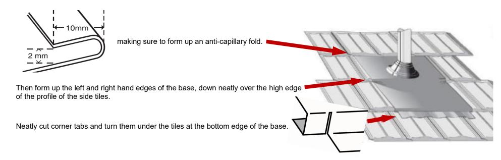
To finish... trim the base to fit or as required to help fit neatly in with the size and profile of the tiles. Make sure you don't over-cut the base and reduce the best result for providing a waterproof membrane over your roof.
