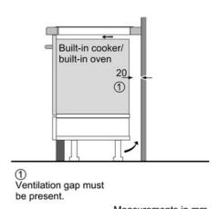
Measurements in mm
